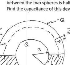
3. A spherical capacitor consists of a spherical conducting shell of radius b and charge -Q concentric with a smaller conducting sphere of radius a and charge Q. The space between the two spheres is half-filled with a dielectric material of strength  $\kappa$  as shown. Find the capacitance of this device.
