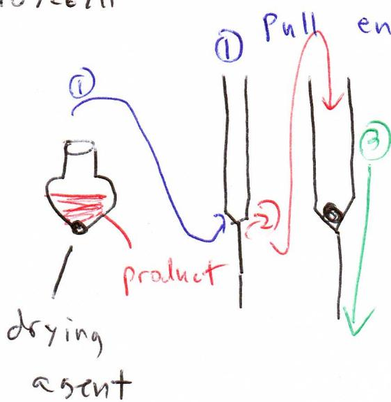
① Pull entire contents of the product flask out using a non-filter pipette
