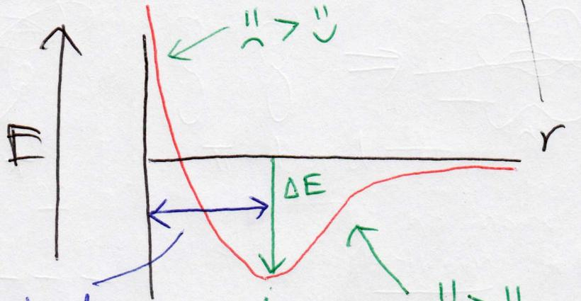
This classical model of bonding is able to describe  $H_2$ , but it fails to describe  $He_2$  because it treats electrons as particles and does not take into account their wave behavior.
