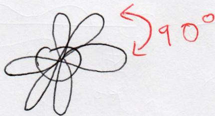
The atomic orbitals of carbon cannot directly be used to describe the molecule methane since the geometry of the orbitals is incorrect and energy of the orbitals is not the same. To describe methane, a set of hybrid orbitals is created by adding and subtracting atomic orbitals on the same atom (LCAO).
