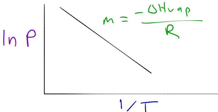
From a set of temperatures and vapor pressures of ethanol, the graph above can be constructed. The slope of this graph has physical meaning.
