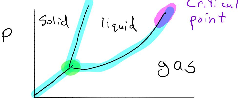
The lines/curves on the diagram represent pressure/temperature combinations in which phases of matter are in equilibrium.
