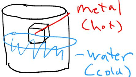
$$q_r = 0 = q_{\text{metal}} + q_{\text{H}_2\text{O}}$$
