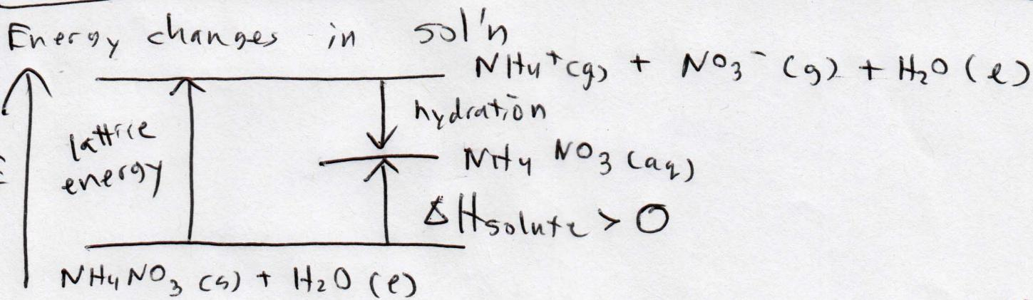
When ammonium nitrate dissolves, the temperature of the solution drops because more energy is necessary to separate the ions (lattice energy) than the energy released by the ions being surrounded by water (hydration).
