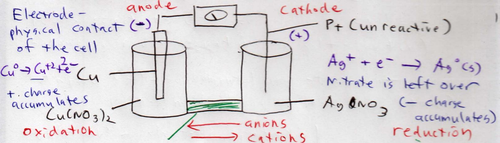
Salt bridge - contains a non-reactive salt (one that will not be oxidized or reduced) that acts as a source of cations and anions to balance the charges generated by the cell
