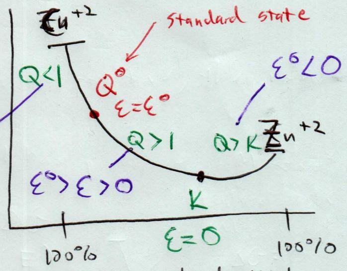
$$\begin{aligned} @25^\circ\text{C} \quad \epsilon &= \epsilon^0 - \frac{0.0592}{n} \ln Q \\ &= \epsilon^0 - \frac{0.0592}{2} \ln (5.0 \times 10^{-5}) = 1.23 \text{ V} \end{aligned}$$
