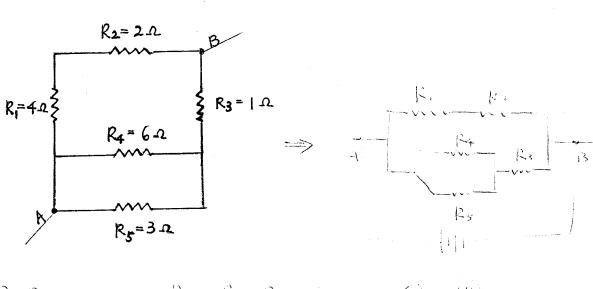
R<sub>1</sub> R<sub>2</sub> in series. R<sub>12</sub> = R<sub>1</sub> + R<sub>2</sub> = 421 + 22 = 62. (6)
