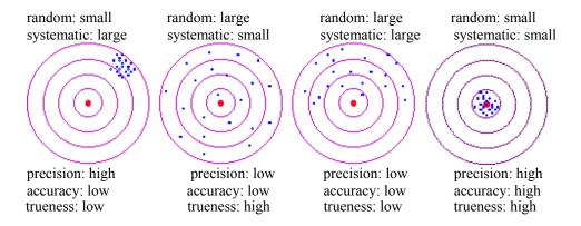
Trueness — a measure of the closeness of the mean of a set of measurements to the exact (true) value.
