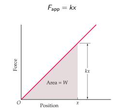
What is the work done by the applied force in stretching the spring a distance x?
