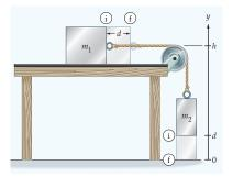
System: Masses  $m_1$  and  $m_2$ , modeled as point particles, and the Earth.
