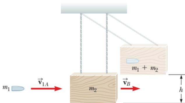
The ballistic pendulum is an apparatus used to measure the speed of a fast-moving projectile such as a bullet. A projectile of mass  $m_1$  is fired into a large block of wood of mass  $m_2$  suspended from some light wires. The projectile embeds in the block, and the entire system swings through a height  $h$ . How can we **determine the speed of the projectile** from a measurement of  $h$ ?
