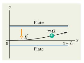
A charge particle follows a parabola, because the field is **uniform**.
