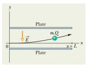
The displacement in the vertical (y) direction (same dir. as field lines)
