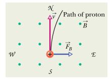
The force on the particle is  $\perp$  to its velocity and the field.
