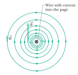
How to determine the direction of the field lines (right-hand rule):
