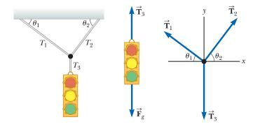
Find the tensions  $T_1$  and  $T_2$ .
