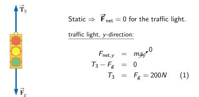
Example: A traffic light weighing 200 N is suspended by two light cables, as shown in the diagram, so that  $\theta_1 = 30^{\circ}$  and  $\theta_2 = 45^{\circ}$ .
