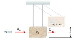
The ballistic pendulum is an apparatus used to measure the speed of a fast-moving projectile such as a bullet. A projectile of mass  $m_1$  is fired into a large block of wood of mass  $m_2$  suspended from some light wires. The projectile embeds in the block, and the entire system swings through a height h. How can we **determine the speed of the projectile** from a measurement of h?
