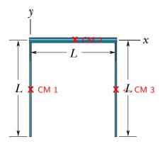
If an object is made up of several different regular shapes, you can find the center of mass by treating each part as point mass at the center of mass of that shape.
