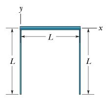
If an object is made up of several different regular shapes, you can find the center of mass by treating each part as point mass at the center of mass of that shape.
