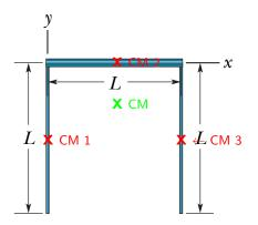
Suppose this 2-D object, plate *P*, has uniform mass-per-unit-area. How can we find its center of mass without integrating?
