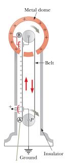
Can (in principle) build up to 3 million Volts when used in air.
