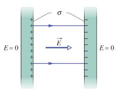
The potential difference between the two plates, separation, d:
