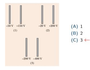
Consider three pairs of parallel plates with the **same separation**. The electric field between the plates is uniform and perpendicular to the plates.
