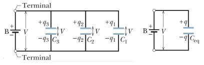
We could replace all three capacitors in the circuit with one equivalent capacitance. The current and potential difference in the rest of the circuit is unchanged by this.
