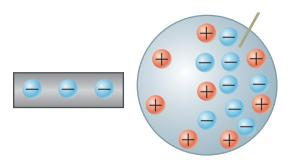
A (negatively) charged object is brought close, polarizing the conductor.
