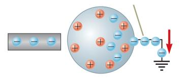
Excess (negative) charge on the far side is drawn off the conductor by grounding it.
