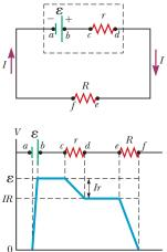
Let  $\Delta V$  be the potential difference supplied by the battery to the rest of the circuit:
