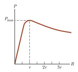
The *y*-axis is the power delivered to the load resistance.
