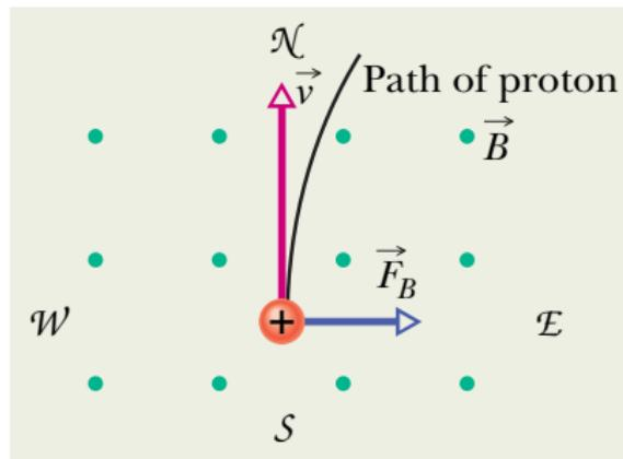
The force on the particle is  $\perp$  to its velocity and the field.
