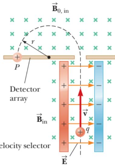
Where they collide with the detector allows us to find the radius of the path,  $r$ .
