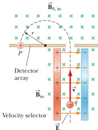
Where they collide with the detector allows us to find the radius of the path,  $r$ .
