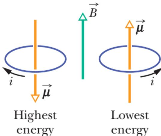
The energy can be found by integrating the torque over the angle of rotation, choosing  $U(\pi/2) = 0$ . (See Lecture 13 for derivation.)
