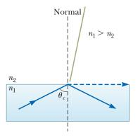
In this case, the angle of refraction  $\theta_2 = 90^{\circ}$ .
