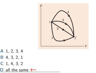
The figure shows four paths on a p-V diagram along which a gas can be taken from state i to state f. Rank the paths, greatest to least, according to
