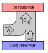
This type of process, where work is converted into a heat transfer from a colder object to a hotter one is called a **heat pump**.
