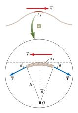
We can use the force diagram to find the force on a *small* length of string  $\Delta s$ :
