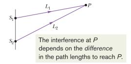
This is because the path difference will correspond to a phase offset of the arriving waves at P:
