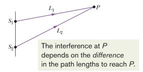
The sound will be louder at different points, depending on the difference in the path lengths that the sound waves take.
