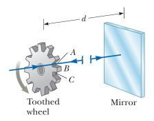
The teeth broke up the beam into pulses as it rotated.
