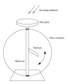
Even very intense light at a low frequency will not allow the plate to discharge. As soon as just a little light at a high frequency falls on the plate it begins discharging.
