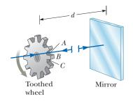
Assume Fizeau's wheel has 360 teeth and rotates at 27.5 rev/s when a pulse of light passing through opening A is blocked by tooth B on its return. If the distance to the mirror is 7500 m, what is the speed of light?
