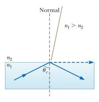
In this case, the angle of refraction  $\theta_2 = 90^{\circ}$ .
