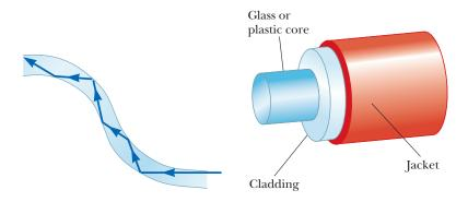
Optical fibers are mainly used for telecommunications: much more information can be carried by an optical fiber than an electrical one in a given amount of time.
