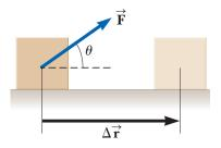
For a constant force applied at an angle  $\theta$  to the direction of the displacement of the block Work is defined as:
