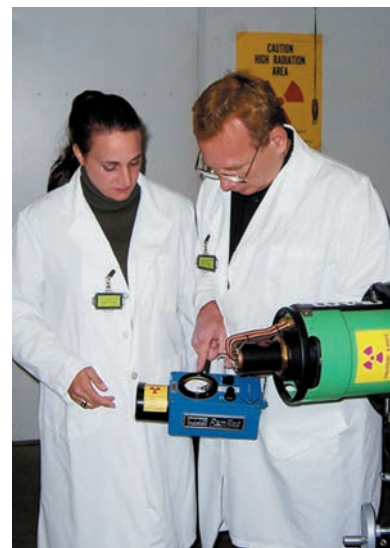
FIGURE 33.9 The film badges worn by Tammy and Larry contain audible alerts for both radiation surge and accumulated exposure. Information from the individualized badges is periodically downloaded to a database for analysis and storage.
