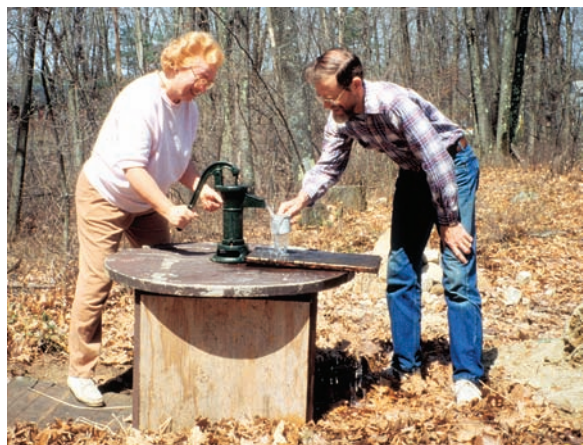
FIGURE 14.9 The atmosphere pushes water from below up into a pipe that is partially evacuated of air by the pumping action.
