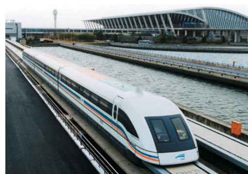
FIGURE 24.11 A magnetically levitated vehicle—a magplane . Whereas conventional trains vibrate as they ride on rails at high speeds, magplanes can travel vibration-free at high speeds because they levitate above the guideway.
