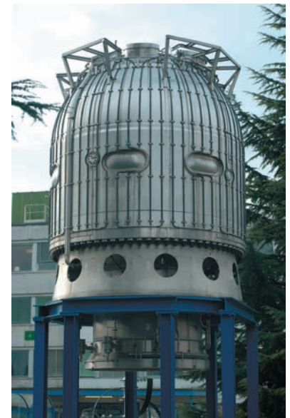
FIGURE 33.21 The Big European Bubble Chamber (BEBC) at CERN, near Geneva, typical of the large bubble chambers used in the 1970s to study particles produced by high-energy accelerators.
