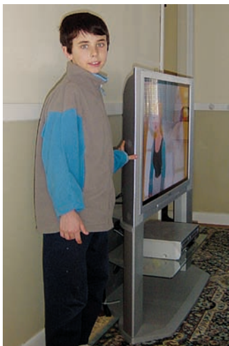
FIGURE 14.26 In a plasma TV, hundreds of thousands of tiny pixels are lit up red, green, and/or blue by glowing plasmas. These colors are combined in different proportions to produce the entire color spectrum.
