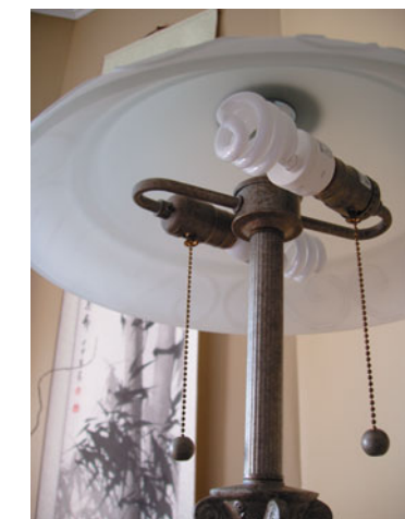
FIGURE 30.16 This pair of 23-W CFLs emit as much light as a pair of 100-W incandescent lightbulbs operating at the same voltage.
