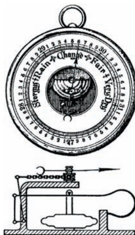
FIGURE 14.10 An aneroid barometer (top) and its cross-section (bottom).
