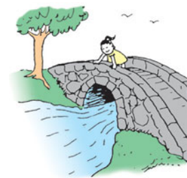
FIGURE 14.16 Because the flow is continuous, water speeds up when it flows through the narrow and/or shallow part of the brook.
