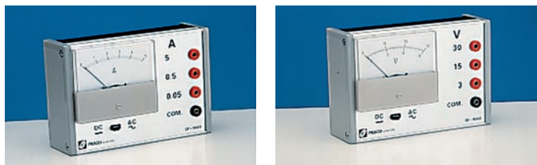
FIGURE 24.18 Both the ammeter and the voltmeter are basically galvanometers. (The electrical resistance of the instrument is made to be very low for the ammeter and very high for the voltmeter.)
