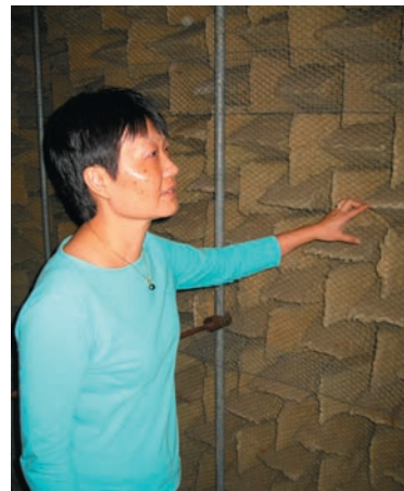
FIGURE 20.7 Special spongy walls absorb rather than reflect sound in this acoustical quiet room.
