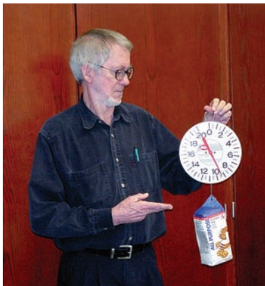
FIGURE 2.13 Burl Grey, who first introduced the author to tension forces, suspends a 2-lb bag of flour from a spring scale, showing its weight and the tension in the string of about 9 N.
