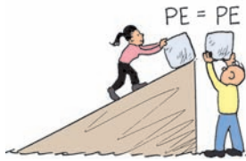
FIGURE 7.8 Both do the same work in elevating the block.
