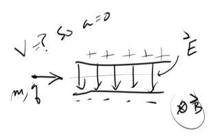
3. Mass spectrometer: From the diagram, a charge q is injected with a known velocity into the region. With the diameter measured as D, find the mass of the charge.
