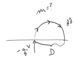
4. From the diagram, find the increase in kinetic energy after the charge makes one full cycle around the cyclotron.
