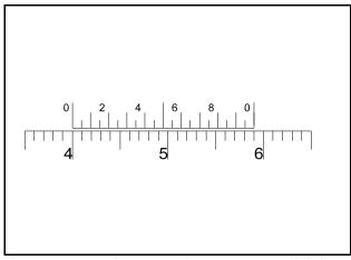
Figure 5: The calipers you will use have 20 divisions in the space of 19. The scale ratio is 20:19.
