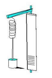
2. Increase the mass of the hanging weight and measure the resultant change in the position of the pointer against the mirrored background ruler provided with the apparatus. Use the mirror qualities of the ruler to align the actual pointer to the image of the pointer in the mirror. by
