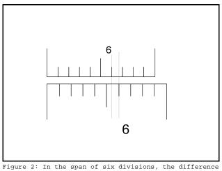
Figure 2: In the span of six divisions, the difference between the vernier and main scale is 0.6 divisions.
