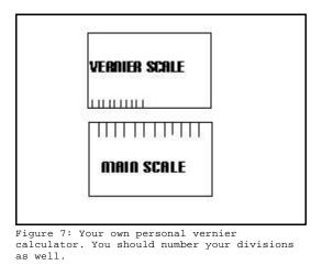
4. You have made your first (and last?) vernier scale which will measure an interpolation of the main scale to a tenth of a centimeter (one millimeter). For one more significant figure, you could interpolate the vernier scale as well.
