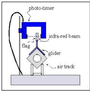
The correct position of the photogate and cart. End View
