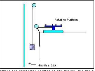
Ignore the rotational inertia of the pulley, but don't forget to include the increasing kinetic energy of the hanging mass as it falls.
