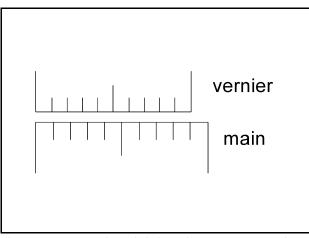
Figure 1: Ten vernier divisions in the space of nine main scale divisions, a scale ratio of 10:9.
