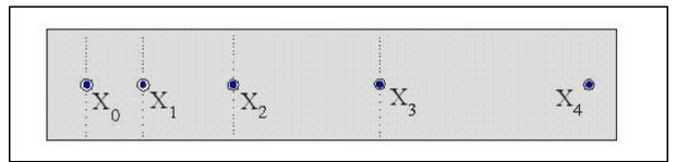
Figure 1: Circle every sixth dot for a total of five circled dots. The time interval between every sixth dot is 6 X 1/60 of a second or 1/10 of a second.
