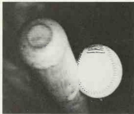
figure 10-1 A high-speed flash photograph of a bat striking a baseball. Notice the deformation of the ball, indicating the enormous magnitude of the impulsive force at this instance. (Courtesy Harold E. Edgerton, Massachusetts Institute of Technology, Cambridge, Mass.)
